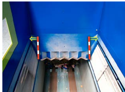
Pre-press side flaps extend the feed opening with minimal height increase
